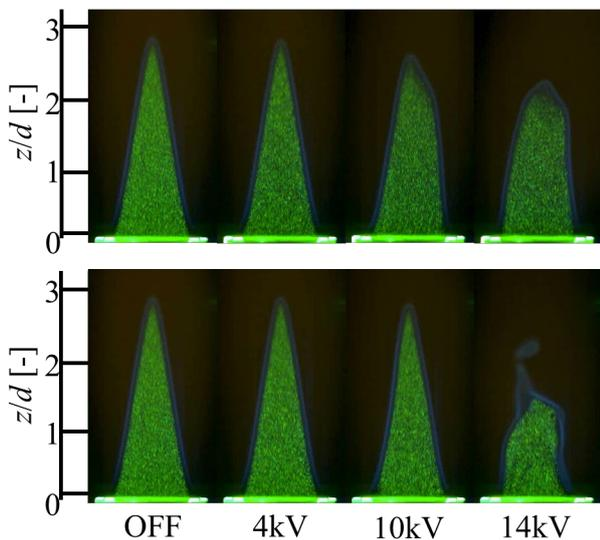
Fig. 5 Comparison of flame visualization
