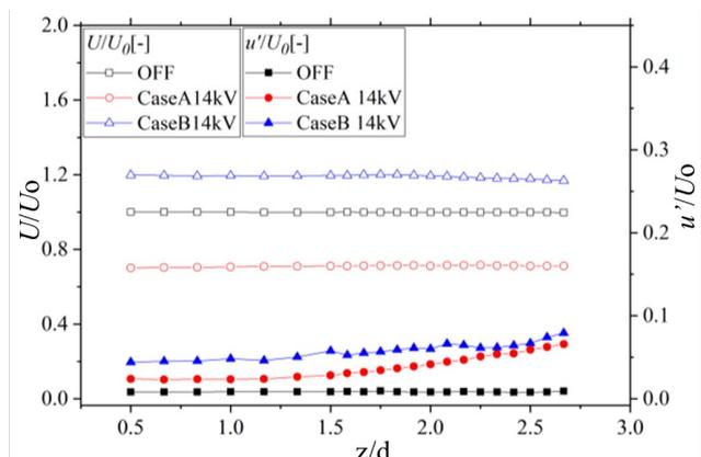
Fig. 8 Jet velocity and turbulence on the center axis of nozzle
